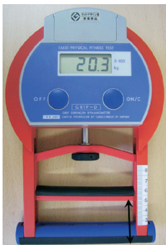
FIGURE 2: Device for measurement of grip span (0.1-cm precision).
